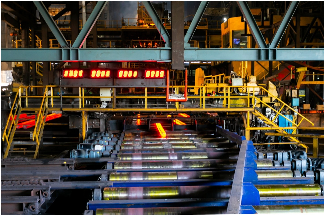
Masteel's Direct Casting and Direct Rolling process cuts carbon intensity by eliminating fossil fuels in billet heating
